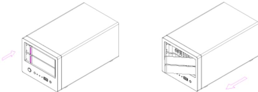
Install the hard drive, making sure the connector is facing the open side of the bracket. Slide the tray back into the enclosure and push the handle lightly into place.
