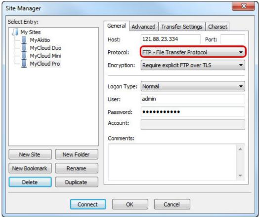
6. For the encryption, select **Use plain FTP**. If the FTP server is set to use SSL encryption, select **Require explicit FTP over TLS** instead.
