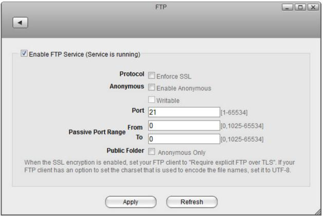
4. If you plan on connecting remotely from outside your home network, it's best to enable the option **Enforce SSL** and to assist port forwarding, it's necessary to set a **passive port range** of about 50-100 ports.
