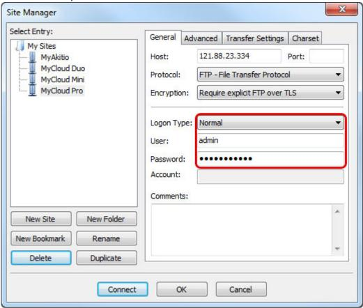
8. Under normal circumstances, these are all the settings you have to configure and the rest can be left at default. However, if you have changed the port number for the FTP server and it's not using the default port 21, remember to enter the correct port number in the FTP client at this
